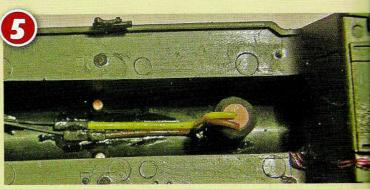
Once you are satisfied that everything will fit back together glue the smoke generator into the chimney of the locomotive body with an epoxy resin and allow to harden. Glue the wires in place too and create the connections to the decoder.
