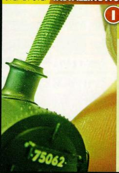
The first stage with this part of the project is to separate the body from the chassis as detailed in the manufacturer's instructions. With this done the moulded chimney needs to be opened out to accept the smoke generator. Do this slowly and carefully removing only a small amount of material at a time. Constantly test fit the smoke generator until it is a snug fit inside.
