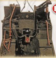
A red LED installed into the firebox hole. You can just make out the black insulated wires from the front locomotive lamp in addition to those I soldered to the LED. They are routed away from possible contact with chassis and glued in place.
