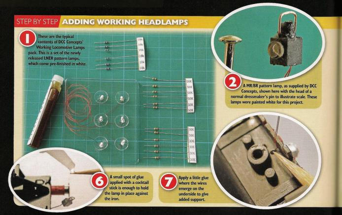
to the point where they will connect to the locomotive wiring, making sure they will not rub against any other components. If this is not possible, you may need to create some space using a fine file.
