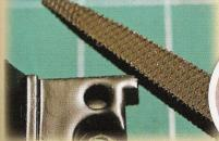
Check the wire routing. If there is likely to be any chaffing of the LED wires, make a bit of clearance on the chassis with a warding file.
