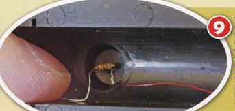
The inside of the dome on the BR '4MT' makes a good clear space to locate the necessary resistor This will be insulated before final re-fitting.
