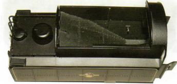
With the coal removed from the bunker the detail and the lack of space can be clearly seen. The general layout of Hornby's DCC equipped interior is neat but cramped.
