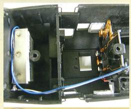
I fed the wires across the cab, holding them in place with mastic. I used colour coded wires so the polarity would be dear when I no longer could see the SC68.
