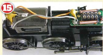
This view shows the general disposition of the DCC fitting components and motor wiring. The amber coloured suppression capacitors play no useful role in a DCC fitted model but can interfere with smooth running in some cases, so I removed them.
