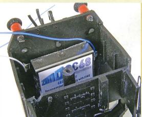
The SC68 now fits comfortably within the bunker, so I secured it in place with a small spot of mastic.
