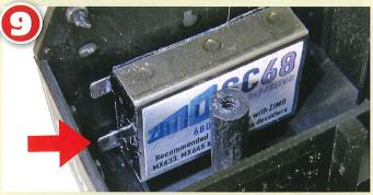
A test fitting of the SC68 showed the lower connecting tab to be preventing the capacitor from seating correctly, probably interfering with the refitting of the weight.
