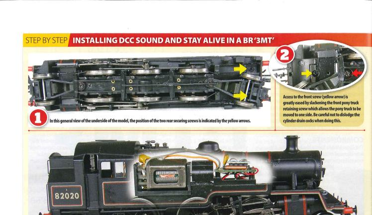
Viewed from the outside, this cutaway shows the available space inside the Bachmann '3MT' bodyshell. There isn't a huge amount of space due to the metal weights either side of the motor, but with careful selection of components a full sound installation with totally hidden features is possible.
