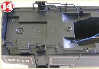
Rigidity was restored when the weight was fixed in place with the three screws and a few drops of cyano type adhesive in the relevant places. The body was set aside whilst the work moved onto preparing for the decoder and speaker installation.
