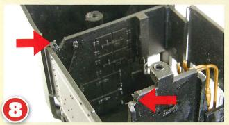
To allow wires from the bunker to pass across the cab footplate without getting pinched, I removed a little plastic from the areas indicated, cutting a 'V' shape to accommodate the wires.
