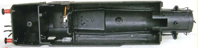
The bunker is only lightly fixed to the rear of the cab roof and without the weight screwed and glued in place the body is severely weakened so much care will be required. If the two parts become detached, some liquid solvent can be applied to join them together later. Here the space inside the coal bunker can be seen.
