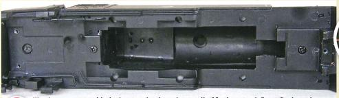
When the screws are removed the chassis, motor and gearbox can be removed by sliding them out vertically, revealing the metal weight and the space available forward of the motor and gearbox. Remove the three screws along the centreline. If you do not intend to fit a stay alive capacitor, jump to Step 15.
