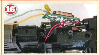
The DCC socket takes up far too much of the available space. After releasing the single screw at the leading edge, it can be moved to one side. Detaching the track and motor wires allows complete removal.
