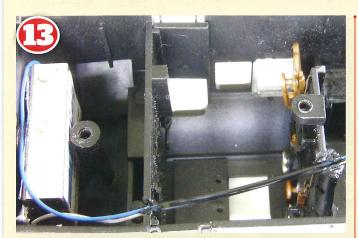
Through the open cab area I painted these wires matt black all around to complete their disguise on the cab floor, but left the free ends in their original colours to identify the positive and negative leads.
